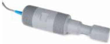
The Sensaphone Toroidal Conductivity Sensors are used in processes where conventional contacting sensors may become fouled or corroded. These probes are unique in the marketplace. They are loop-powered and provide direct 4-20 mA output. (Part # FGD-0070)
