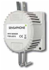
The Sensaphone FGD-L8215 Spot Type Liquid Leakage Detector is used to detect the presence of liquid on a horizontal surface. High Voltage and Current Rating of the Dry Contact Relay Output allow FGD-L8215 Spot Type Liquid Leakage Detector to control electrical solenoid water valve directly. Green LED indicates the power of the device is on while Blinking Red LED indicates the detection of liquid.
