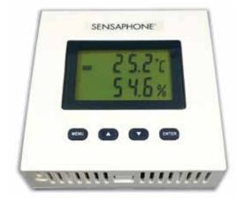
The Sensaphone FGD-0109 Dual Sensor is a compact and user friendly temperature and humidity sensor. It measures and displays both ambient temperature and relative humidity at the same time. Two 4-20mA analog outputs are available.
