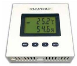
The Sensaphone FGD-0108 Dual Sensor is a compact and user friendly temperature and humidity sensor. It measures and displays both ambient temperature and relative humidity at the same time. All configuration is stored in the system's non-volatile memory. Two Normally Open (NO) solid state outputs are available.
